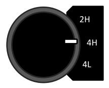
To engage 4x4, simply turn the 4WD dial from 2H to 4H. This can be performed while driving at speeds less than 70km/hr. A message will appear on the dash reading "4x4 shift in process". The shift itself will take a few moments to engage and you can proceed to drive as normal.
